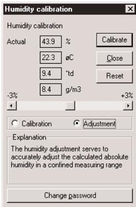
The second window (activate by setting the button to Adjustment) in **HUMIDITY CALIBRATION** is not an alternative for adjustment. However, it provides the option of moving the characteristic curve parallel in a small working range, if the data is correct at the calibration points (11.3 or 75.3 %RH  $\pm$  2 %RH) to, for example, superimpose the calculated values (dew point and absolute humidity) with a reference instrument.
