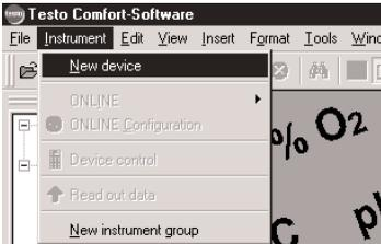
Activate the instrument driver for the testostor 171 data logger series in **INSTRUMENT / "NEW DEVICE"** and click on the "Next" button.
