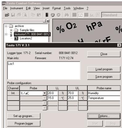
Here is the example of a programmed logger.
