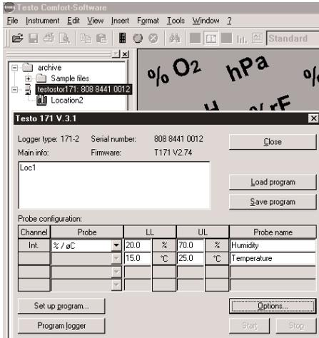
Connect the logger to the PC and open the main instrument window. Select the HUMIDITY CALIBRATION window in **OPTIONS**. The measured *Actual values* are shown in the additional window which appears. When the *Actual value* is stable, confirm with the 11.3 % button so that the calibration is saved directly in the probe/instrument, the old calibration data is discarded and the actual value shows 11.3%. Repeat the process with the 75.3% RH container (adaption time is also 30 min to 1 h).
