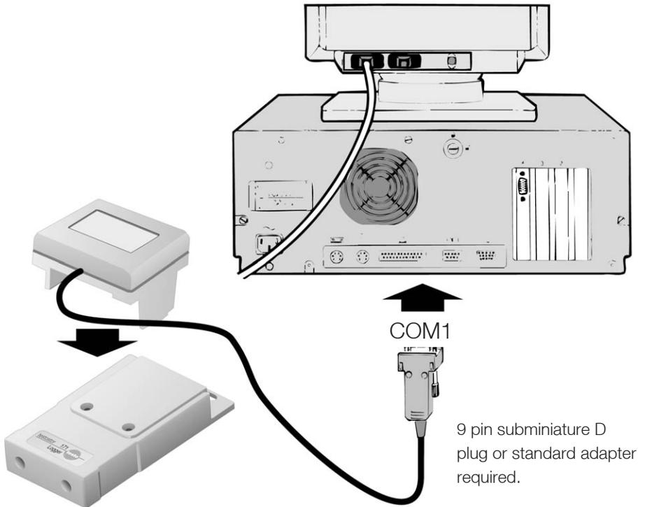
To program or read your data logger, the interface connected to the computer is plugged into the data logger.
